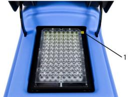
Figure 3. Correct microplate placement. 1. "A1" symbol for microplate alignment
