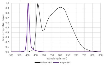
Figure 4. Relative spectral power in relation to wavelength for photodiodes (white and purple led maximum spectral power are not equal)
