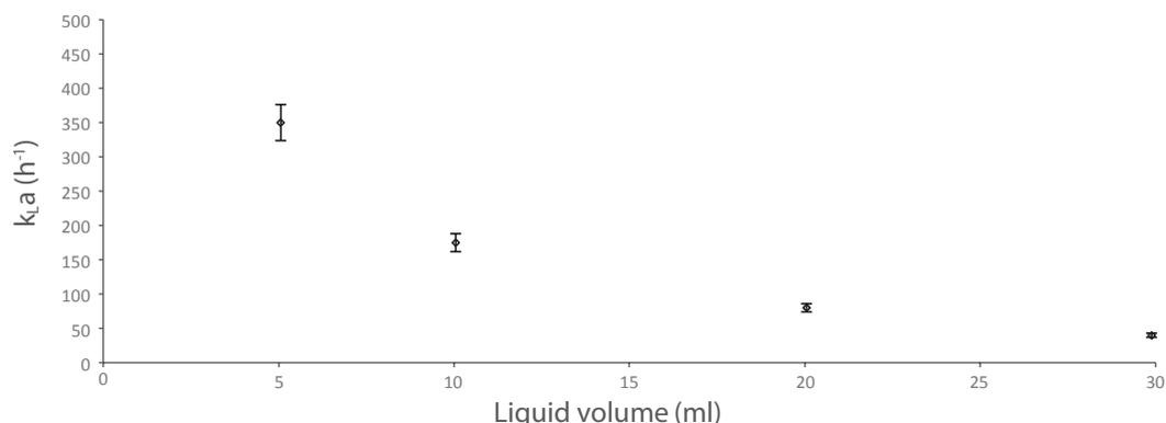
Figure 9. Determination of  $k_{L,a}$  in 50 ml TPP Bioreaktor tubes. The bioreaktor vessels were filled with 5, 10, 20, 30 ml deionized water and measurements were made by non-invasive  $O_2$  sensors and optics (PreSens, Regensburg, Germany) at 30 °C using a gassing-out method. Mean and standard deviation of at least five independent experiments are shown.
