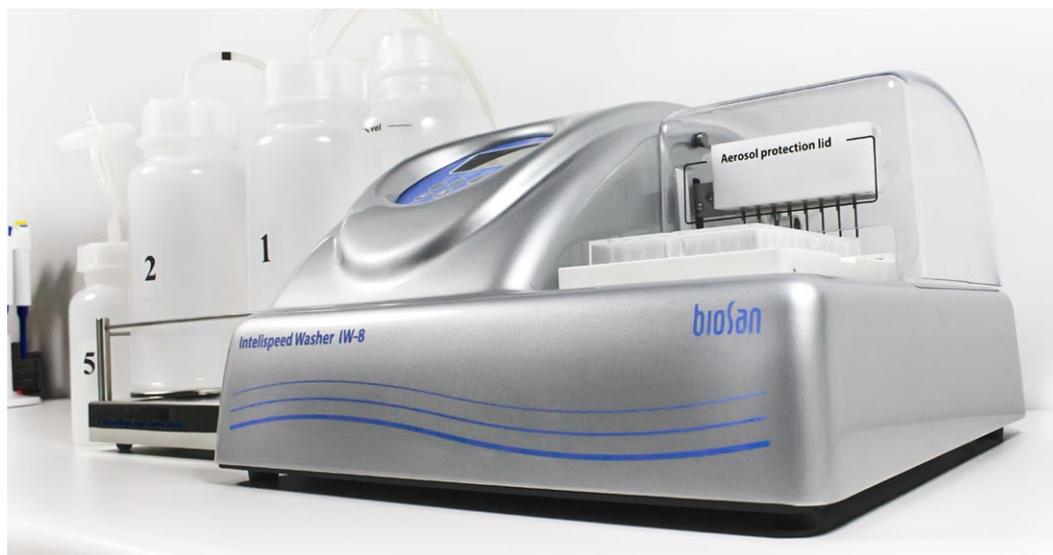
4-channel washing solution weight logger, **4 CHW Logger** provides automatic control of rinsing solutions and waste volume. The washer shows the remaining volume for each bottle as a percentage and gives a warning message in case of low solution volume or full waste bottle when **4 CHW Logger** is connected.
