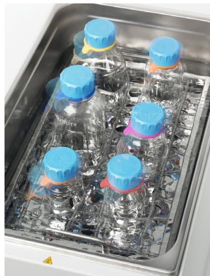
Patented, combined orbital and linear shaking mechanism of the **OLS26** allows optimisation of aeration and shear forces mixing for reproducible results.
