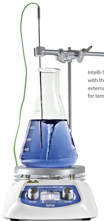
Intelli-Stirrer MSH-300i with the stand, external probe and holder for temperature probe
