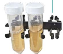
PRS series platforms are equipped with universal rubber clamps for different size tube fixation; PRSC series platforms have metal clamps able to hold heavier solutions (e.g. soil, sand).
