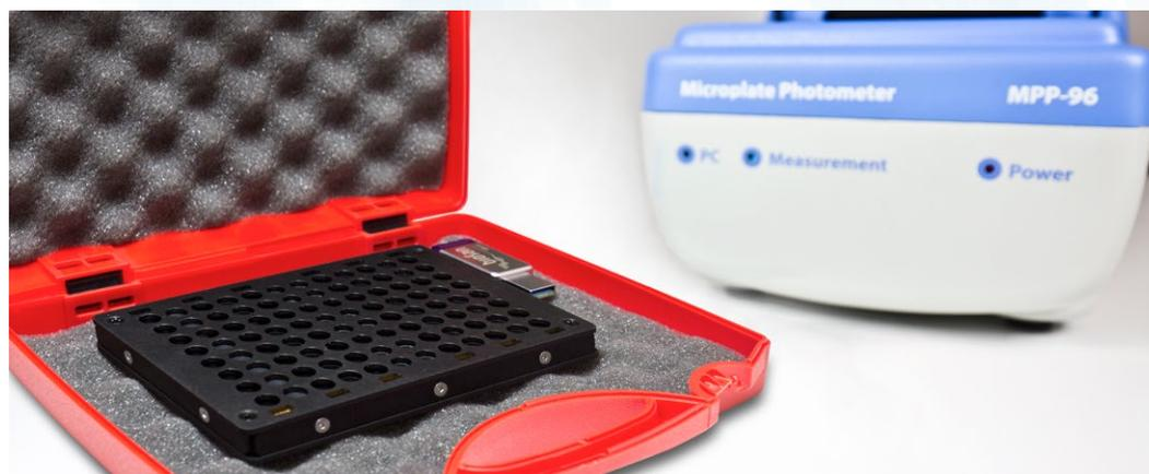
**DESCRIPTION** **OD Plate** is the measurement verification instrument for microplate photometer MPP-96 HiPo. The instrument is designed to verify the accuracy and precision of measurements of the photometer at six levels of nominal optical density: 0.3; 0.6; 1.0; 2.0; 3.0; 4.0 OD. The instrument is supplied with the following verification wavelength range: 405–700 nm.
