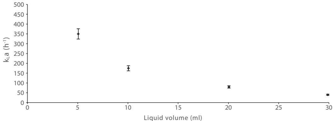
Figure 3. Determination of  $k_{i,a}$  in 50 ml TPP Bioreactor tubes. The bioreactor vessels were filled with 5, 10, 20, 30 ml deionized water, and measurements were made by non-invasive O<sub>2</sub> sensors and optics (PreSens, Regensburg, Germany) at 37°C using the gassing-out method. Mean and standard deviation of at least five independent experiments are shown.
