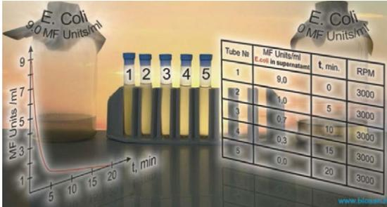
Application of **DEN-1** for determining microbial cells concentration of supernatant in tubes during centrifugation. Turbidity is determined in McFarland units.
