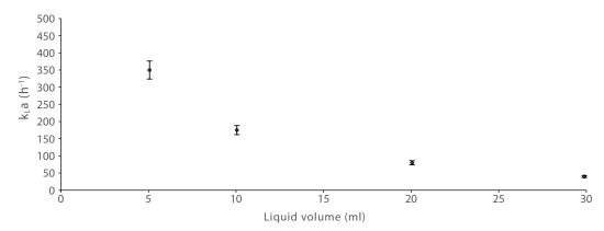
Figure 3. Determination of  $k_L$ a in 50 ml TPP Bioreactor tubes. The bioreactor vessels were filled with 5, 10, 20, 30 ml deionized water, and measurements were made by non-invasive  $O_2$  sensors and optics (PreSens, Regensburg, Germany) at 37°C using the gassing-out method. Mean and standard deviation of at least five independent experiments are shown.
