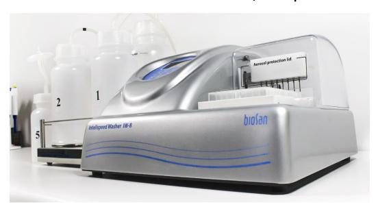
4-channel washing solution weight logger, 4 CHW Logger provides automatic control of rinsing solutions and waste volume. The washer shows the remaining volume for each bottle as a percentage and gives a warning message in case of low solution volume or full waste bottle when 4 CHW Logger is connected.
